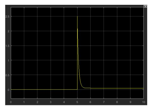
The Simscape Component block points to an ideal capacitor component. Simulation results show that, when the switch is flipped at t=5 seconds, the capacitor delivers 2.5 A to the load.
