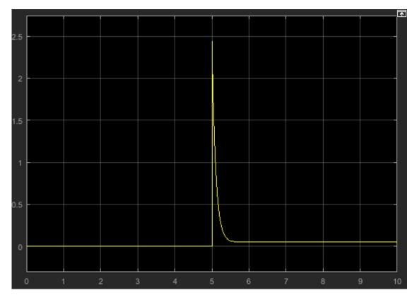
Simulation results show that, when the switch is flipped at t=5 seconds, the current delivered to the load is less than 2.5 A.
