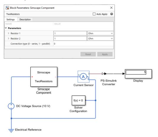
If you change the value of the **Connection type (0 - series, 1 - parallel)** parameter to 1, the resistors are connected in parallel, and the current is 20A.
