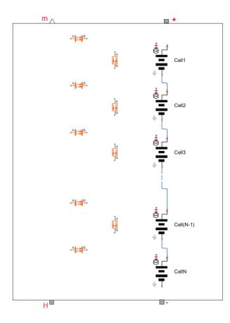
Then connect this internal chain to the two electrical nodes of the composite component:
